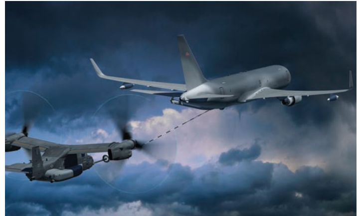
The NewGen Tanker is shown refueling a V-22 Osprey from the centerline hose unit.
